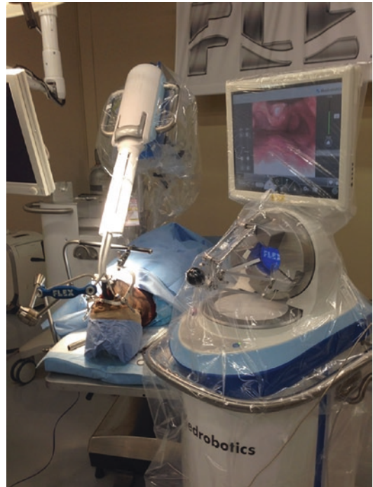
Fig. 7.1 Medrobotics Flex robot, approved for transoral robotic surgery in 2015
