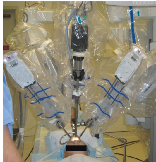
Fig. 7.2 Da Vinci robot setup with endoscope in the center and instruments on each side oriented at 45° from the center camera
