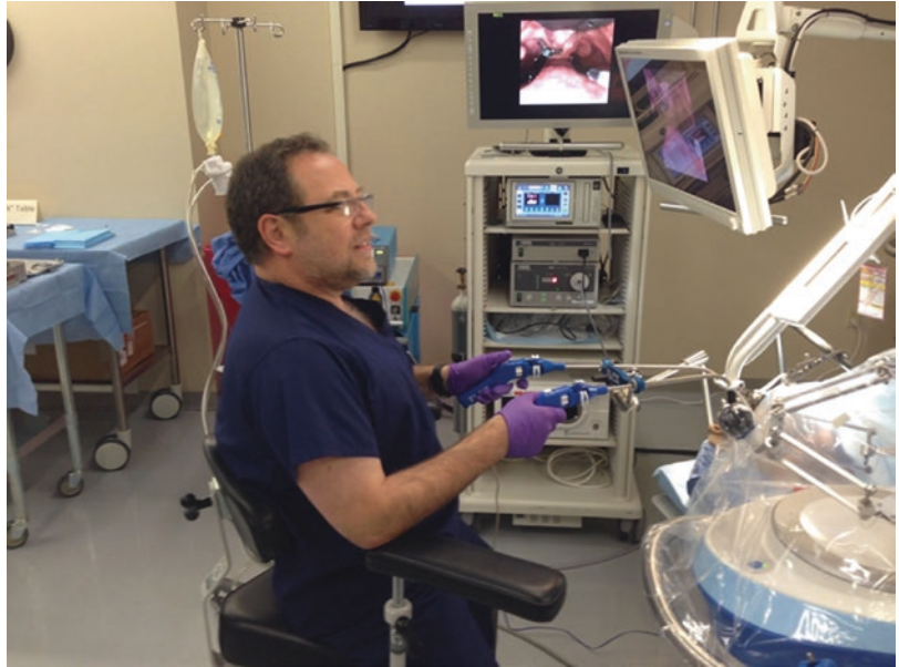
Fig. 7.3 Medrobotics Flex robot mounted to patient bed rails with surgeon at the patient's head controlling instruments
