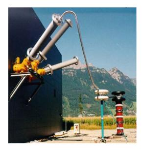
**Fig. 22.2** Gas-insulated test transformer and coupling capacitor for PD measurement directly connected to the GIS
