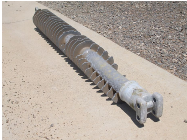
Fig. 40.2 Extreme bird damage of a composite insulator (Australia)
