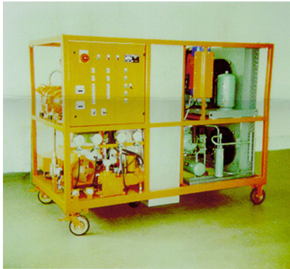
Fig. 27.32 Gas handling device pump and gas mixing unit
