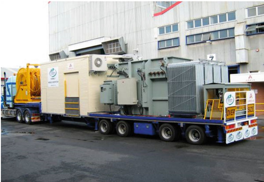
Fig. 6.9 The “NOMAD” mobile substation includes cable reels for rapid connection to pre-prepared substations (courtesy Ergon Energy, Australia)
