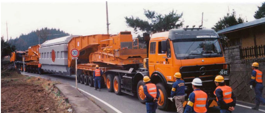
Fig. 28.7 Transportation of UHV transformer to the site in Japan
