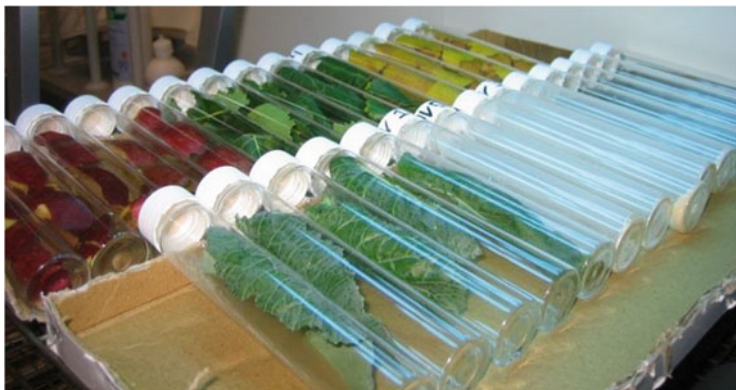
Fig. 6 Plant leaves inserted in UV-B transparent vials. Note vials without leaves are used as blank controls
