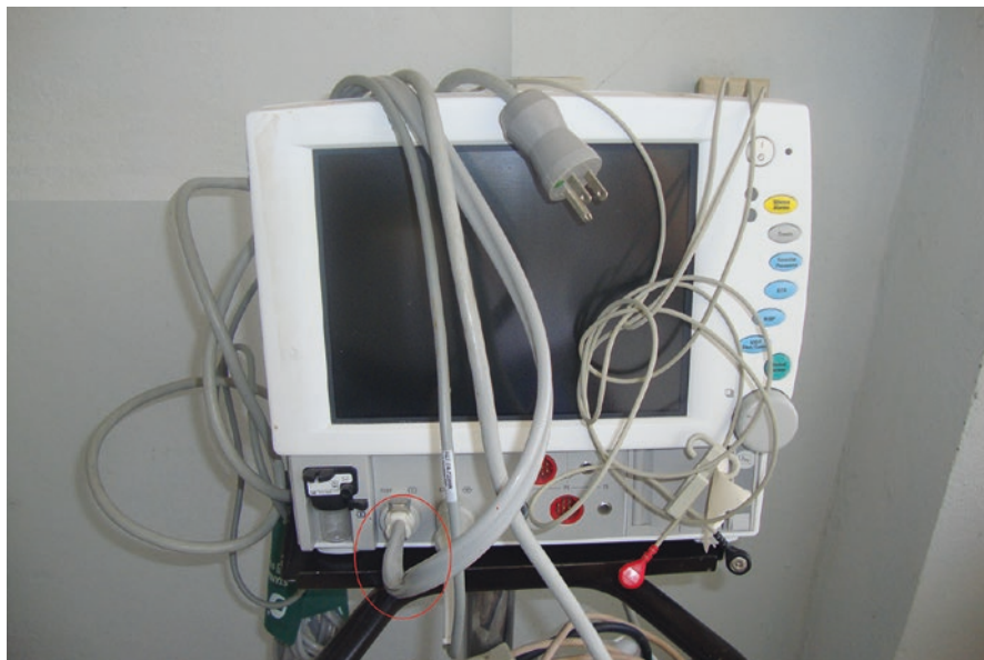
Fig. 10.7 This is not the correct care and handling of patient accessories. Note the kinked blood pressure hose near the connector
