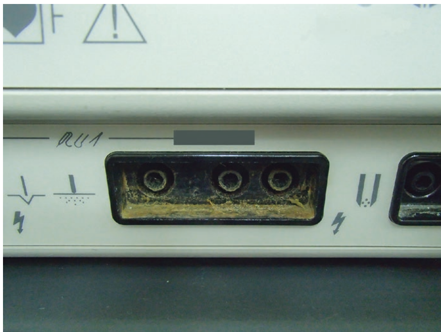
Fig. 10.6 This electro-surgical unit/Bovie pencil connector was damaged from an improper cleaning solution
