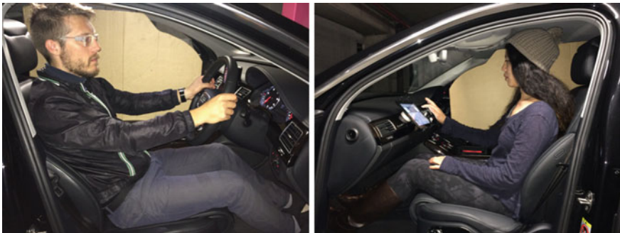
Fig. 18.9 AutoRoute Test Setup. Realized as Wizard-of-Oz autonomous car improvised by a cardboard divider. Left picture the driver. Right picture Setup for the study participant with AutoRoute app running on tablet-pc mounted on the passenger's dashboard
