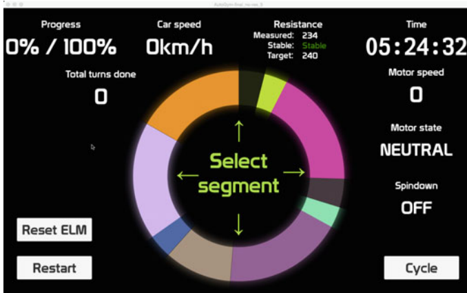
Fig. 18.2 AutoGym graphical user interface. The circle represents the whole exercise program that has to be completed by selecting the segments for workout
