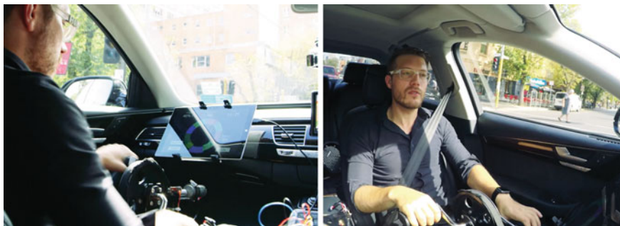
Fig. 18.1 AutoGym play test in the car with manually operated spinning bike and tablet-pc for the game interactions
