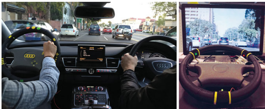
Fig. 18.5 In-car game design session based on a second steering wheel ( left image ). AutoJam prototype in development: each drum or synth sound is assigned to one of the three touch pads with LED indicator ( right image )
