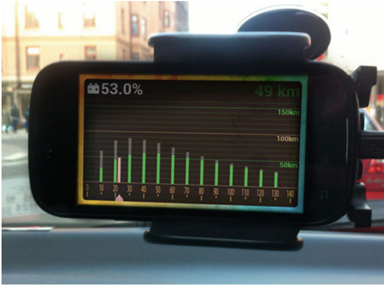
Fig. 5.5 Differentiated Driving Range app showing the correlations between driving speed (current speed just above 20 km/h), driving range and climate control. Grey bars show maximum attainable driving range for different speeds with the climate control turned off. The green bars overlaying the grey bars show estimated driving range with the current climate control setting
