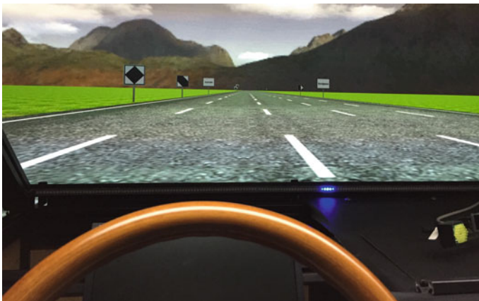
Fig. 7.3 LED visualization of the co-driver's gaze for the driver (driver's perspective)
