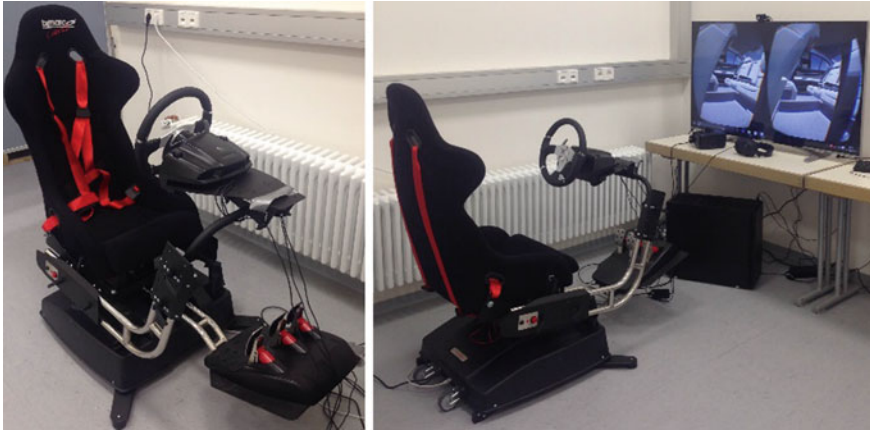
Fig. 15.6 Atomic motion system compact driving simulator
