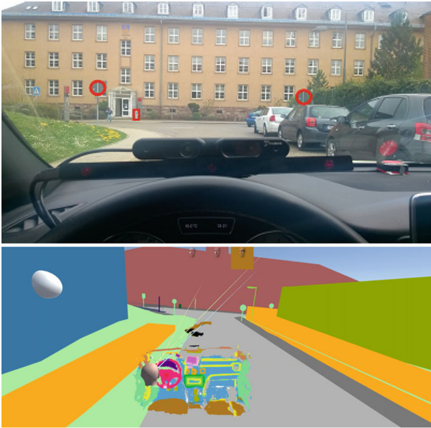
Fig. 9.9 An example scene for precision analysis in outdoor environments containing three target objects. The environment model, the vehicle model, and the direction of the focus are all integrated in one environment. The rays represent the direction of the eye gaze and head pose
