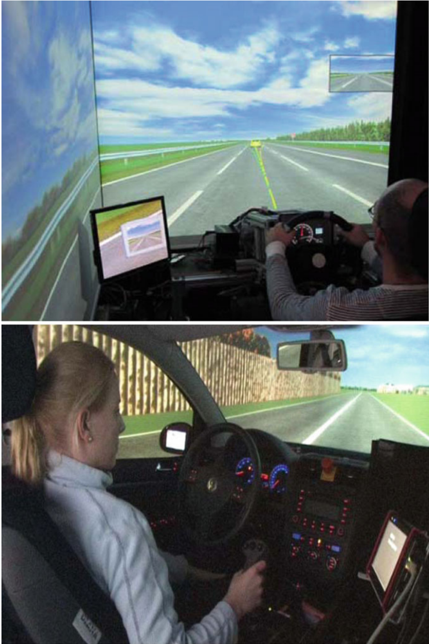
Fig. 3.9 H-Mode with trajectories displayed in the contact analogue head up. Display and active steering wheel/pedal. Application of H-Mode in the dynamic simulator with active sidestick. Flemisch et al. (2014)
