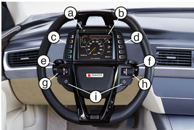
Fig. 13.5 The interactive communication steering wheel iCS, as developed by Audio Mobil and Takata. At the top indicator lamps ( a ) are located. The most prominent element is a touch screen ( b ) visualizing all relevant information. It may also provide an on-screen keyboard. On both sides soft keys ( c , d ) are aligned that dynamically match with functions on the touch screen providing haptic feedback. Behind the steering wheel pull/push elements for light ( e ) and windshield wiper ( f ) interaction are located. Two rotary knobs either operated from the front or from the back allow volume control ( g ) and menu selection ( h ). Turn indicators are implemented as buttons ( i ) on the steering wheel. No instrument cluster or center stack display is needed
