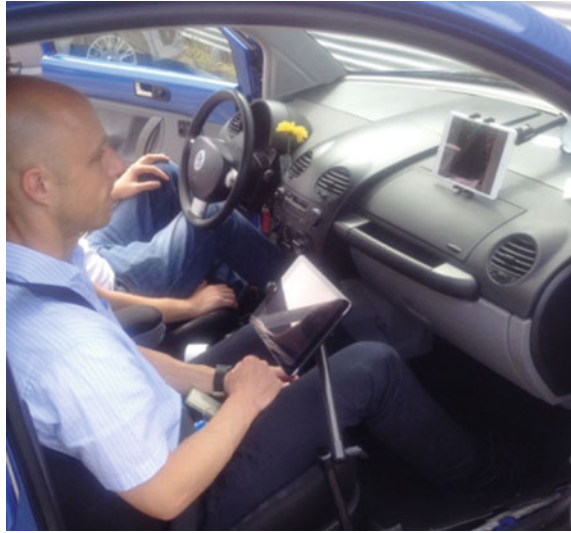
Fig. 17.3 Testing the effect of a higher positioned instrument cluster
