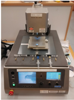
(a) Ultra Tec ASAP-1 polishing machine.
