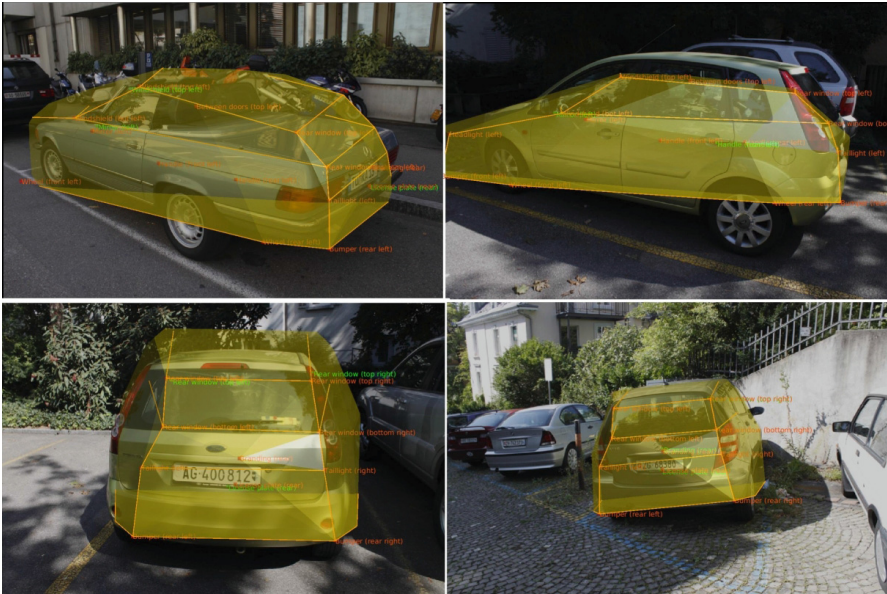
Fig. 7. Qualitative results of the proposed RANSAC-based viewpoint estimation on our dataset, with Viewpoint/Shape estimations overlaid on the object.
