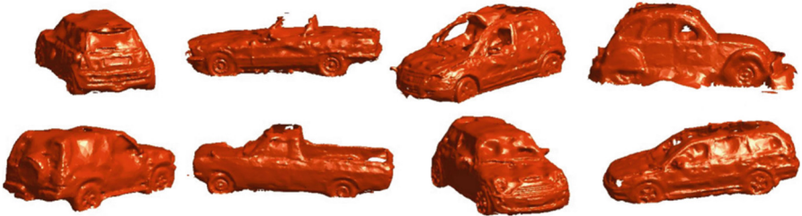
Fig. 2. Training set examples for 'car': 3D meshes obtained from real-world 2D image sequences from 123DCATCH. These models are used for data-driven 3D geometric reasoning throughout the paper. Note the intra-class shape variability.
