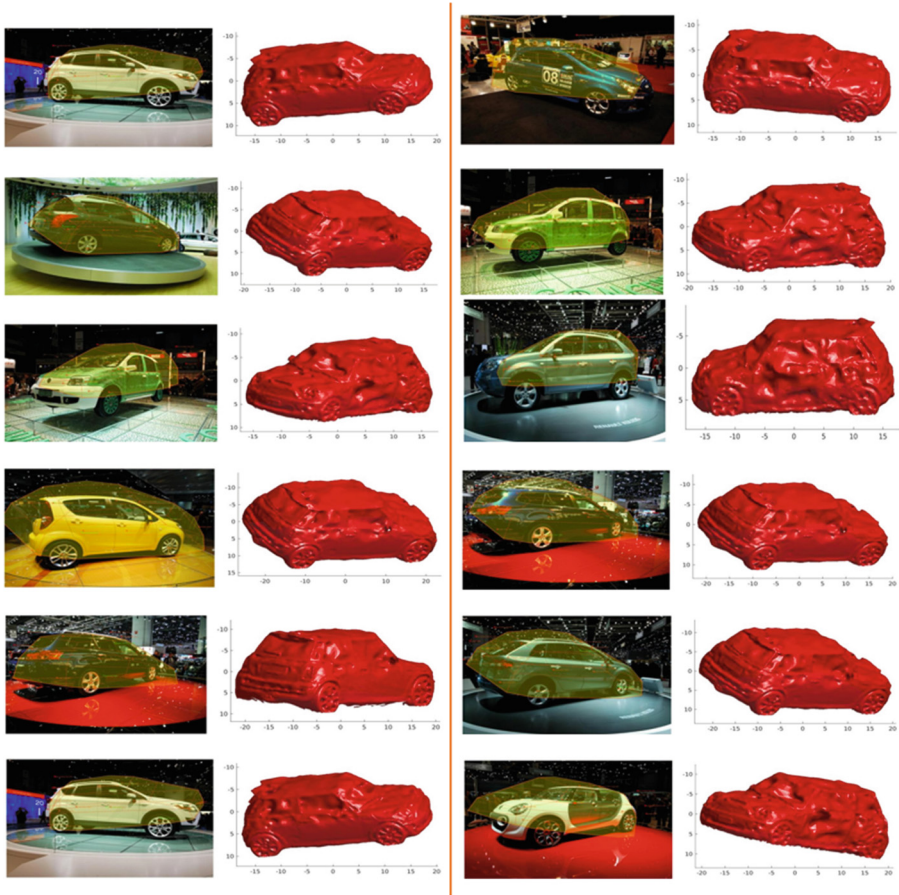
Fig. 5. Qualitative results of the proposed RANSAC -based Viewpoint Estimation and Shape Recovery, on EPFL Multi-view Car dataset. Odd columns illustrate the test image with corresponding Viewpoint/Shape estimations overlaid on it. Even columns illustrate the Viewpoint Estimation of their corresponding test image (on its left), using a sample mesh (from our dataset) for better visualization. ( note: meshes (in even columns) are not generated/reconstructed by our viewpoint estimation approach, and are used only for the purpose of better visualization in all our qualitative results).
