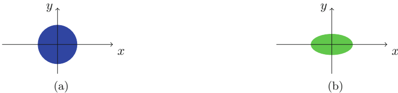
Fig. 4. (a) presents the pictorial representation of the Isotropic correlation in which case symmetric kernel for sampling is required and (b) presents the Anisotropic correlation that prompts the selection of asymmetric sampling kernel
