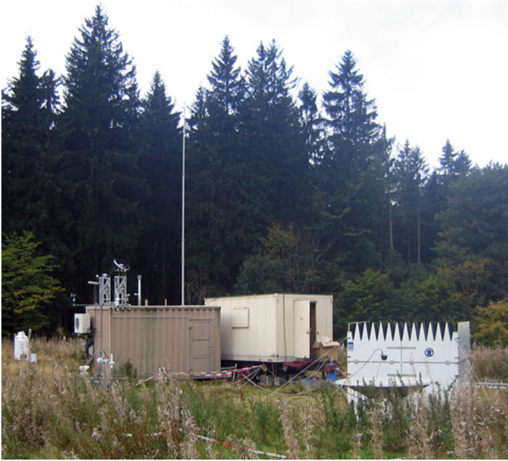
Fig. 2.10 Waldstein-Pflanzgarten site in 2008 with the measurement container (on the top radiation measurements and 10 m wind measurements); in the background the wet-only sampler is visible. Additional instrumentation during EGER-IOP 2 with a measuring container for additional trace gas measurements and a sodar-RASS system in the foreground (2008, Photograph T. Foken)
