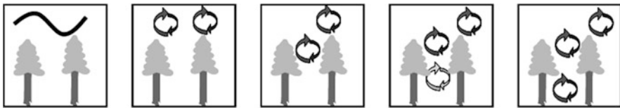
Fig. 6.3 Conceptual depiction of the vertical exchange regimes in order of increasing degree of vertical coupling ( left to right , adapted from Göckede et al. 2007) with kind permission © Authors 2007, CC License 4.0, All rights reserved: Wave motion, Decoupled canopy, Decoupled sub-canopy, Coupled sub-canopy by sweeps, Fully coupled canopy
