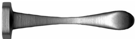
Fig. 5.23 The AE signals waveguide
