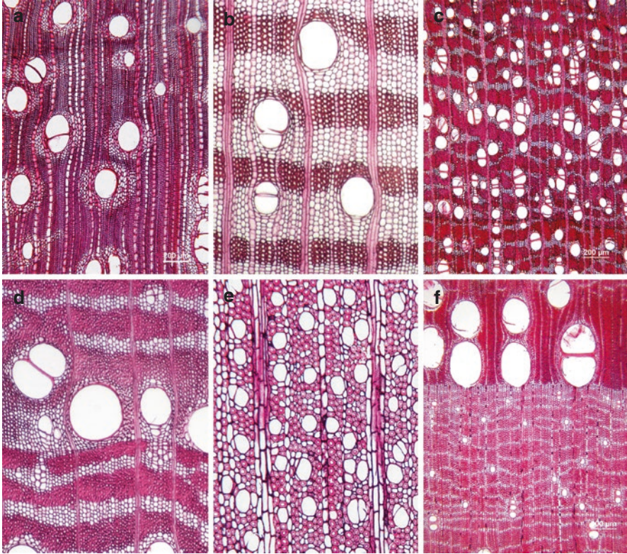
Fig. 7 Transverse sections of angiosperm woods showing a range of axial parenchyma distribution patterns. Parenchyma may ensheath vessels in wide (a) or thin layers (c, f), form tangential bands of varying width and position (b–d, f), or appear in diffuse clusters of one to several cells (e). Parenchyma cells are thin-walled and appear light in color against a background of thicker-walled fibers and vessels. Species shown are (a) Anacardium occidentale [Sapindales/Anacardiaceae], (b) Ficus maxima [Rosales/Moraceae], (c) Celtis ehrenbergiana [Rosales/Cannabaceae], (d) Sapindus mukorossi [Sapindales/Sapindaceae], (e) Viburnum stellatomentosum [Dipsacales/Adoxaceae], (f) Carya ovata var. australis [Fagales/Juglandaceae] (All images courtesy of InsideWood ( http://insidewood.lib.ncsu.edu/ ) and reproduced with permission of the original contributors (Wheeler 2011). Photo credits and copyright: (a, c, e, f) ©Elisabeth Wheeler, North Carolina State University, Raleigh, N.C., USA; (b, d) ©Els Bakker, Naturalis, Leiden, Netherlands)
