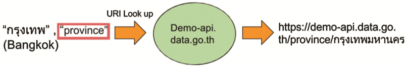
Fig. 3. Example of using semantic type information to resolve word ambiguity in URI lookup
