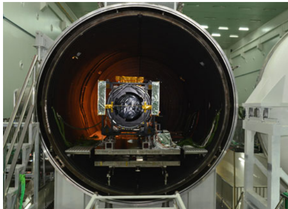
Fig. 12 Thermal vacuum test setup
