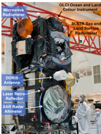
Fig. 1 The Sentinel-3A satellite fully equipped during on-ground testing at Thales Alenia Space, France, in December 2014
