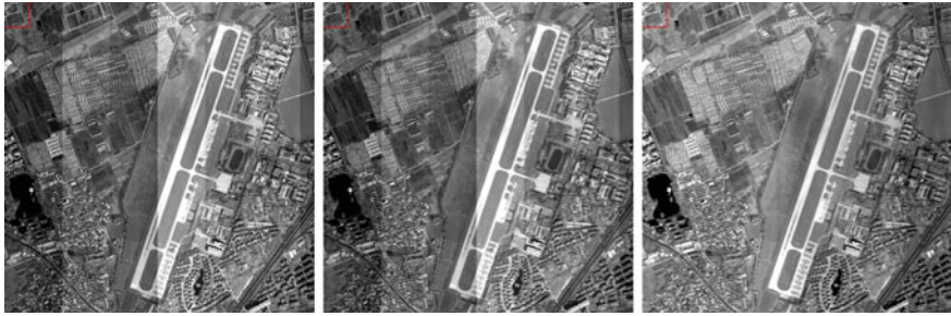
Fig. 8 Left original image of airport; middle airport image correction using lab coefficient; right airport image corection using the coefficient computed from the improved slide-slither method
