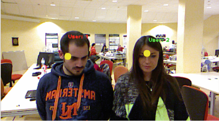
Fig. 1. Users identified by the skeleton tracking and the DRRF (yellow dots). (Color figure online)
