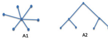
Fig. 1 Two architectures having the same number of nodes and connections but are differentiated based on their internal structure with E(A_1) = 4.9 and E(A_2) = 6.83
