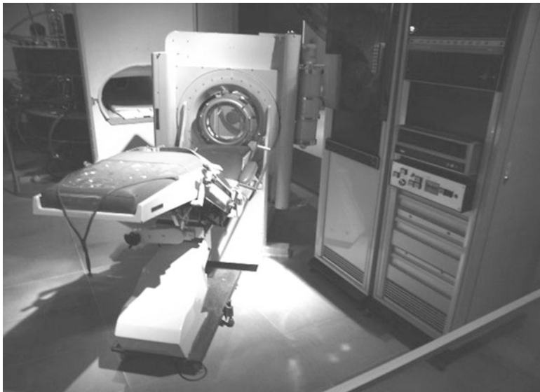
Fig. 27.2 The original EMI head scanner. Source: https://en.wikipedia.org/wiki/CT_scan#/media/File:Emi1010.jpg
