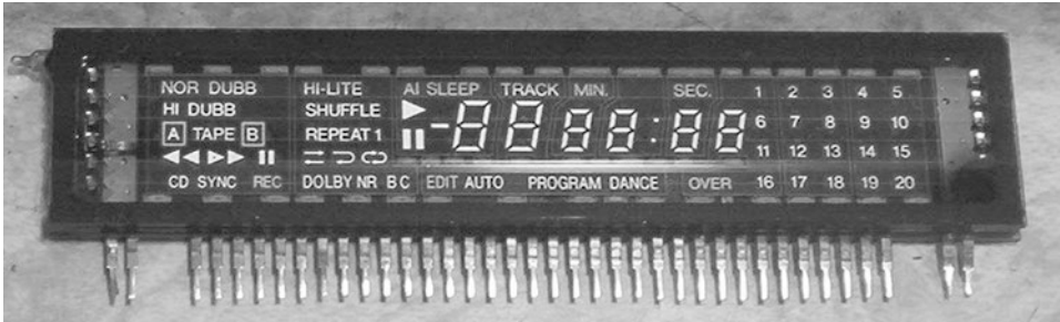
Fig. 12.2 A vacuum fluorescent display showing all the bars and legends, which are a light green color. Source: https://en.wikipedia.org/wiki/Vacuum_fluorescent_display#/media/File:VFD2.jpg
