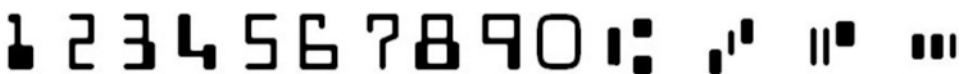
Fig. 24.1 The 14 magnetic ink characters used on cheques so that they could be read by machine. Source: https://en.wikipedia.org/wiki/Magnetic_ink_character_recognition#/media/File:MICR_char.svg
