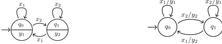
(a) Moore machine M_1 on input-output sets I = \{x_1, x_2\} and O = \{y_1, y_2\} . (b) Mealy machine M_2 on input-output sets I = \{x_1, x_2\} and O = \{y_1, y_2\} .
