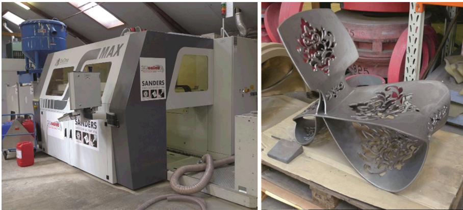
Fig. 6. Large 3D-print installation for the production of massive sand-molds, for cast iron. On the right an example of a complex object, made in one piece, using a single sand mold (installation of the Dutch firm 3dealise)
