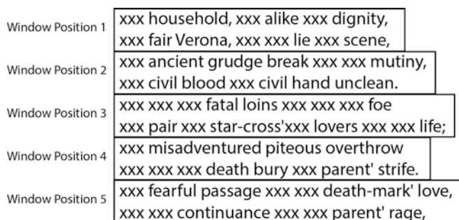
Fig. 5.9 Illustration created to demonstrate how AutoMap creates “windows” to extract word pairs during semantic network generation
