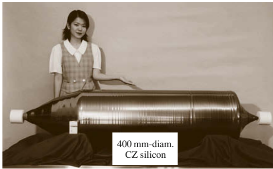
Fig. 13.8 Extra-large as-grown Czochralski silicon ingot 400 mm in diameter and 1800 mm in length. (Courtesy of Super Silicon Crystal Research Institute Corporation, Japan)
