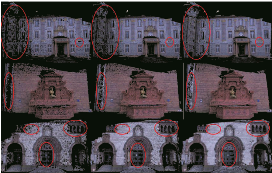
Fig. 5. Datasets from Stecha et al. [15]. From top to bottom row, they are Castle-P10 , Fountain-P11 , Herz-Jesu-P8 . And from left to right column, they are 3D models reconstructed by PMVS, our DAISY-based method and our final method.
