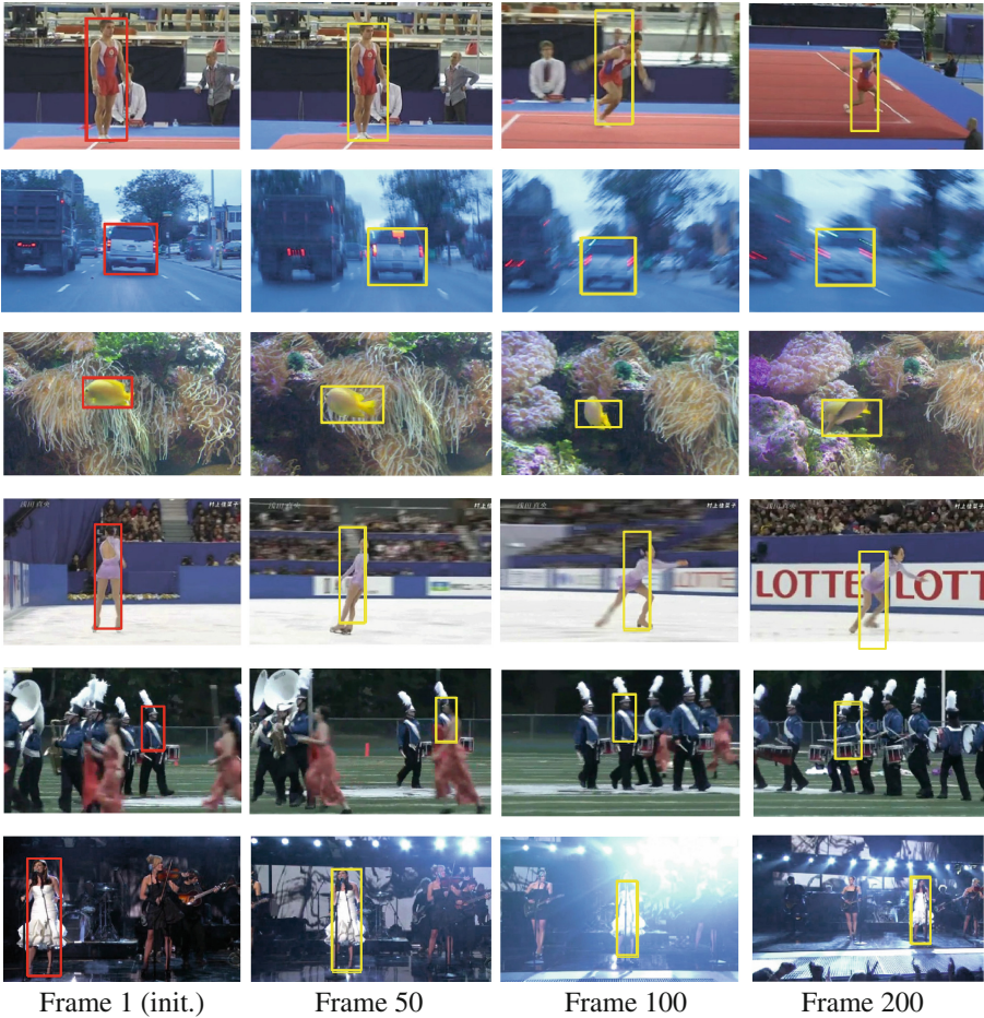
Fig. 6. Snapshots of the simple tracker described in Sect. 2.4 equipped with our proposed fully-convolutional Siamese network trained from scratch on ImageNet Video. Our method does not perform any model update, so it uses only the first frame to compute \varphi(z) . Nonetheless, it is surprisingly robust to a number of challenging situations like motion blur (row 2), drastic change of appearance (rows 1, 3 and 4), poor illumination (row 6) and scale change (row 6). On the other hand, our method is sensitive to scenes with confusion (row 5), arguably because the model is never updated and thus the cross-correlation gives a high scores for all the windows that are similar to the first appearance of the target. All sequences come from the VOT-15 benchmark: gymnastics1 , car1 , fish3 , iceskater1 , marching , singer1 . The snapshots have been taken at fixed frames (1, 50, 100 and 200) and the tracker is never re-initialized.
