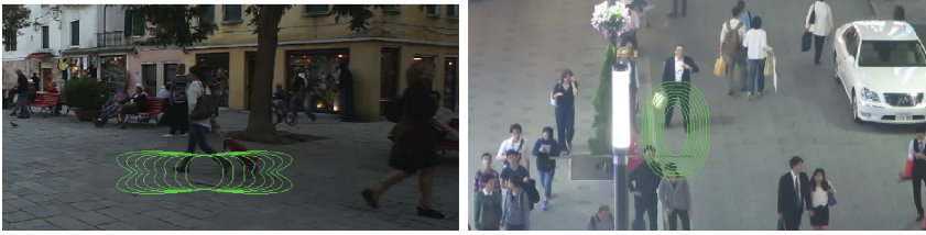
Fig. 2. Position models. The different iso-contours of value 0 of the Potts costs for different values of \Delta (i.e. location of detections occurring after \Delta frames around each shown detection and for which \beta = 0 ), learned from sequences MOT16-01 and MOT16-03. In the region delimited by a curve, association will be favored, whereas outside it will be disfavored. Curves show different moving directions and amplitudes in each sequence.
