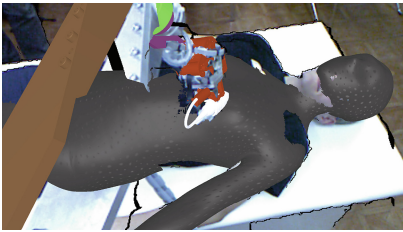
(a) Overlaying the estimated body model with the synchronous Kinect RGB-D stream.
