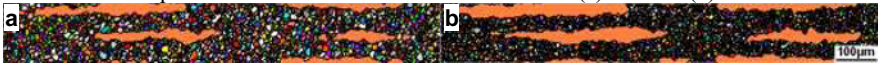
Figure 5. The simulated microstructures with consideration of grain morphology deformation at temperature of 1060^{\circ}C for different strain rates: (a) 0.1s^{-1} and (b) 1s^{-1} .
