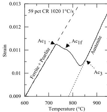
Figure 1. Continuous heating laser dilation vs. temperature curves (strain vs temperatures) for 59 pct. CR 1020 with a heating rate of 1 °C/s.  $Ac_1$  and  $Ac_3$  respectively represent the start and completion of austenite formation.  $Ac_{1f}$  is the pearlite-to-austenite finish temperature [8].
