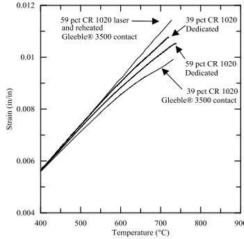
Figure 2. Continuous heating dilation vs. temperature curves for 39 pct. CR and 59 pct. CR 1020 heated at 1 °C/s on a Gleeble® 3500 system and a commercial dedicated push-rod dilatometer. Gleeble data for the 59 pct. CR material are shown for a non-contact laser extensometer superimposed with data on a reheated sample that was fully recrystallized prior to testing.
