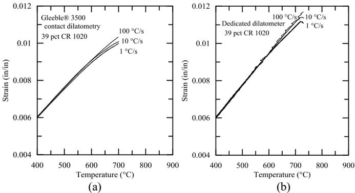
Figure 3. Continuous heating dilation vs. temperature curves as a function of heating rate for 39 pct CR 1020 with (a) Gleeble® 3500 contact dilatometer and (b) dedicated pushrod dilatometer.
