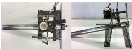
Figure 1. The device for the Inclined Plane Test.
