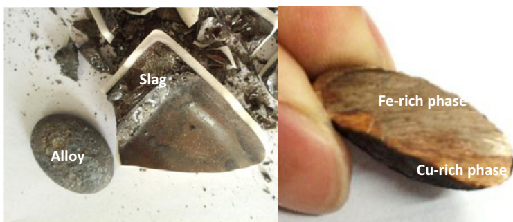
Fig.5 Photographs of smelting products and the immiscibility of alloy without pre-oxidizing roast (smelting for 0.5h at 1350°C)
