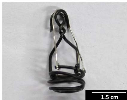
Figure 5. Spinel substrate with spiral shape made by oxidizing iron wire.
