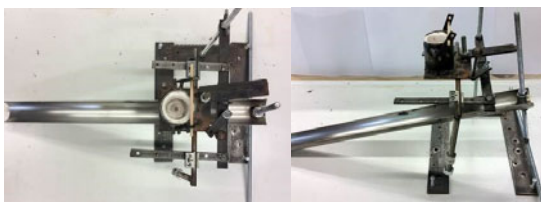
Figure 1. The device for the Inclined Plane Test.
