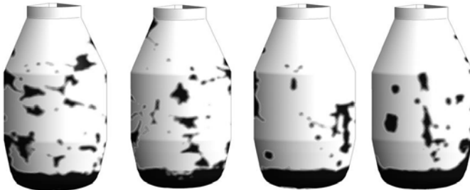
Figure 3: Fraction of slag covering the wall of the converter in time of 2 seconds in the case of kinematic viscosities of (a) 23 \times 10^{-6} \text{ m}^2 \cdot \text{s}^{-1} ; (b) 40 \times 10^{-6} \text{ m}^2 \cdot \text{s}^{-1} ; (left) (c) 200 \times 10^{-6} \text{ m}^2 \cdot \text{s}^{-1} and d) 400 \times 10^{-6} \text{ m}^2 \cdot \text{s}^{-1} (Right); lance to slag distance of 1 \text{ m} , gas velocity of 520 \text{ m/s} ; according to CFD simulation
