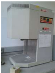
Figure 1. Electric furnace for the fusion process
