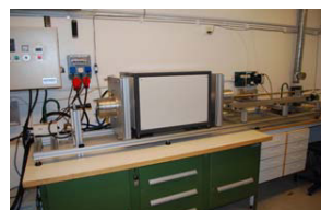
Fig. 2 Experimental setup for contact angle measurements
