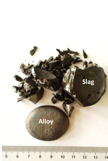
Fig.3 The photograph of smelting product of smartphone PCBs
