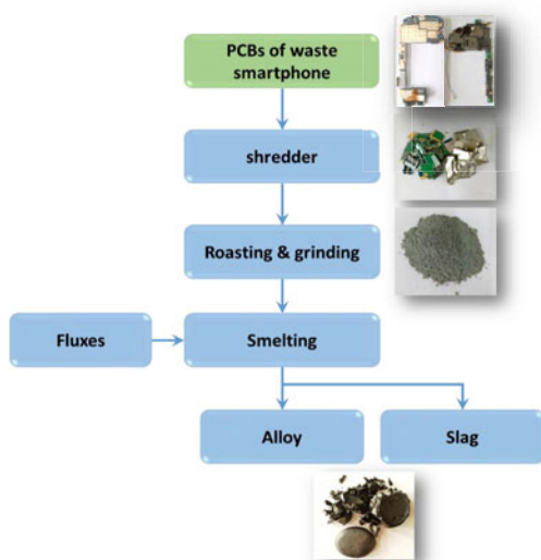
Fig.2 The proposed flowchart of valuable metals recovery from waste smartphone PCBs
