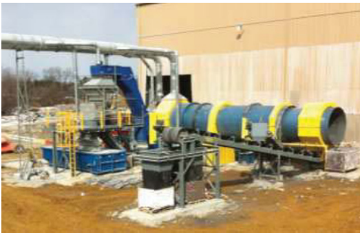
Figure 1. Model RT 108 DIDION Crusher / Metal Separation
