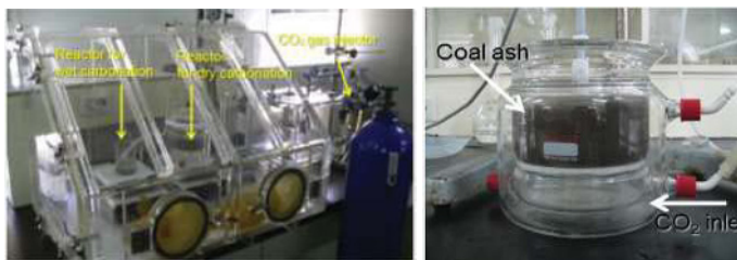
Figure 5. Experimental apparatus of Heavy metals leaching by carbonation method
