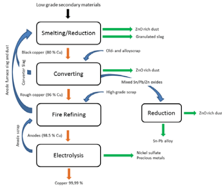
Figure 3: Principle flow sheet of a secondary copper production [9]
