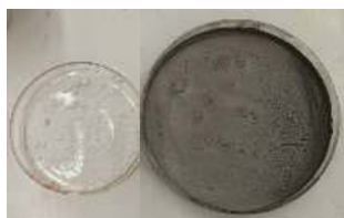
Fig. 2, h-BN powders before (left) and after (right) surface modification
