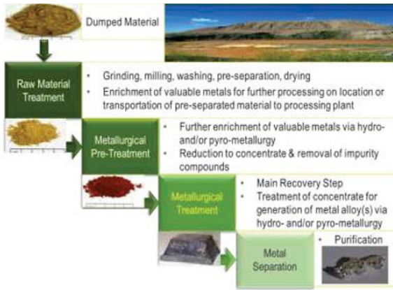
Figure 4: Possible process scheme for multi-metal recovery out of jarosites
