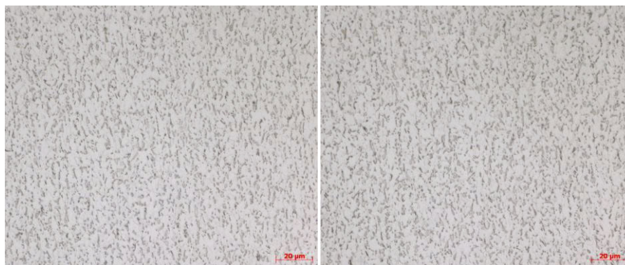
Figure 2 Microstructure (500×) of new rim steel: (a) 1/4 site of sample (b) center of sample
