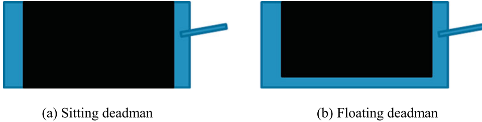
Figure 2. Schematic diagram of deadman state
