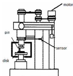
Figure 1. High-temp. face wear tester (MMU-10G)
