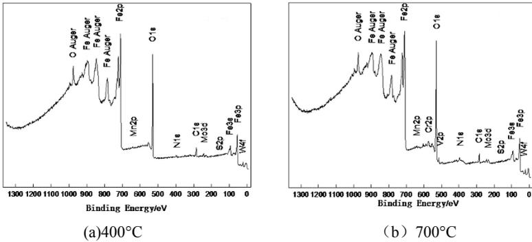
Figure 6. XPS of worn surface
