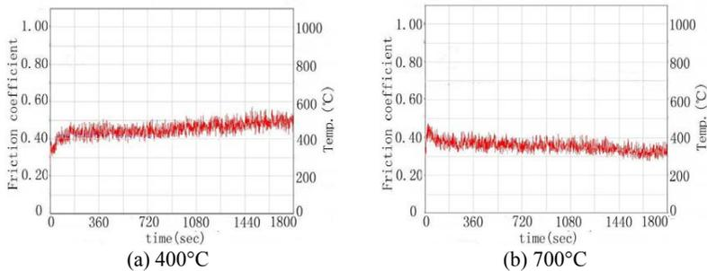
Figure 4. Curves of friction coefficient vs. time at different temperatures
