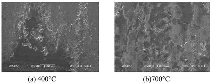
Figure 5. SEM of worn surface
