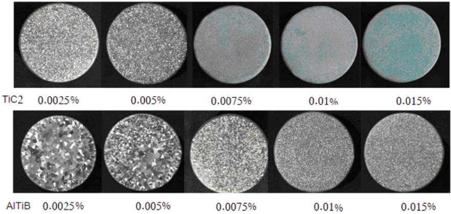
Figure 7. Photomicrographs for the refined commercially pure Al using TiC2 master alloys with different addition ratios.
