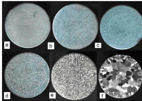
Figure 5. Photomicrographs for the refined commercially pure Al using :
