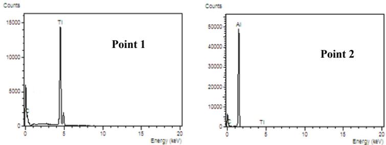
Figure 3. :EDS analysis for the prepared Al-TiC at point 1, 2 indicated above in Fig.2
