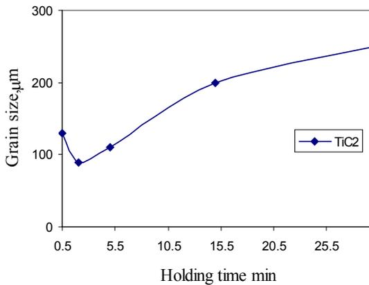
Figure 10. Effect of holding time on the grain size of 99.7 %Al refined with TiC<sub>2</sub> master alloys.
