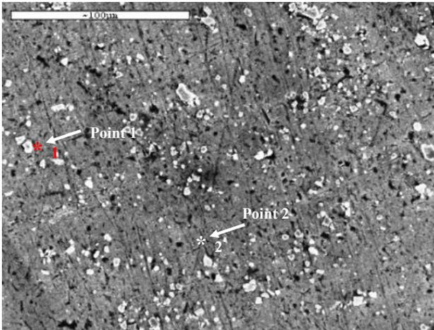
Figure 2. SEM micrograph for the prepared TiC1 containing 3.75Wt.% TiC
