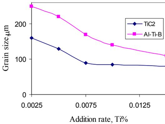
Figure 8. Effect of addition rate on the grain size of the pure aluminum refined with the prepared TiC2 and Al-Ti-B master alloys
