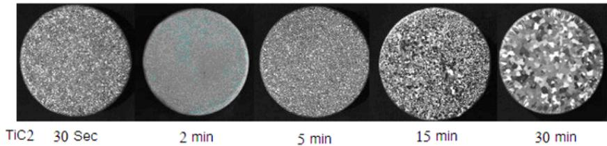
Figure 9. : Photomicrographs for the refined commercially pure aluminum using TiC<sub>2</sub> master alloys with various holding times.
