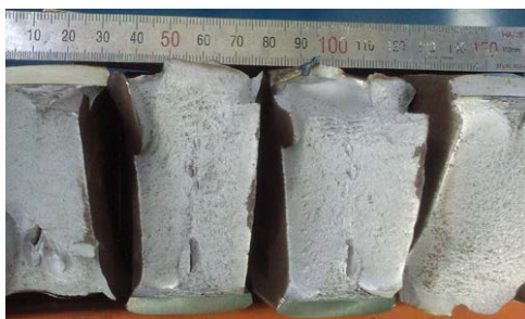
FIGURE 7: DWTT FRACTURE OF X70 PIPE
