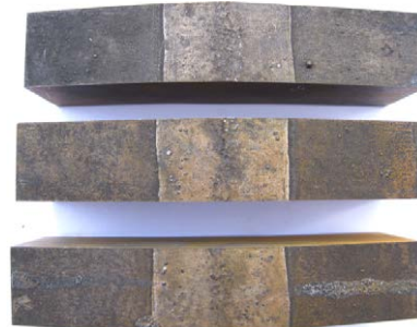
FIGURE9: MACROGRAPH OF WELD MATAL SAMPLE
