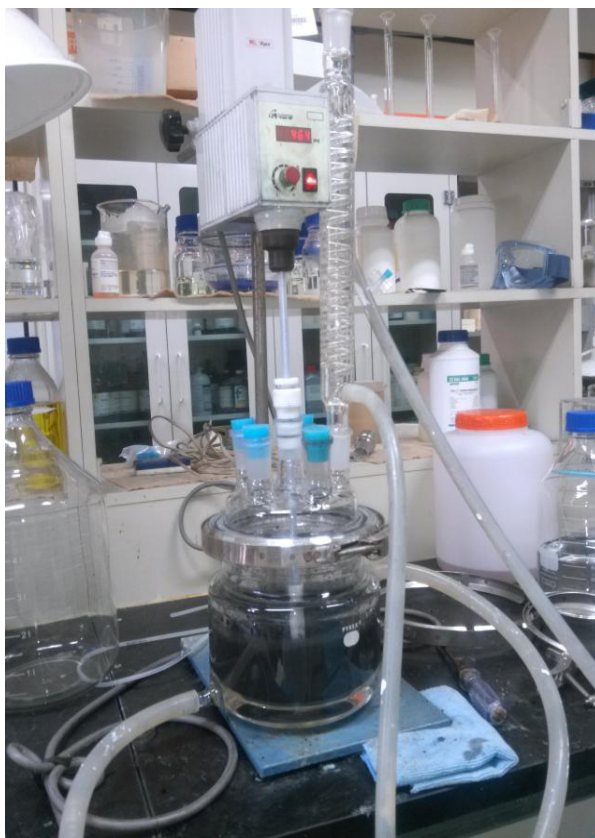
Figure 2. Experimental set up of the leaching process
