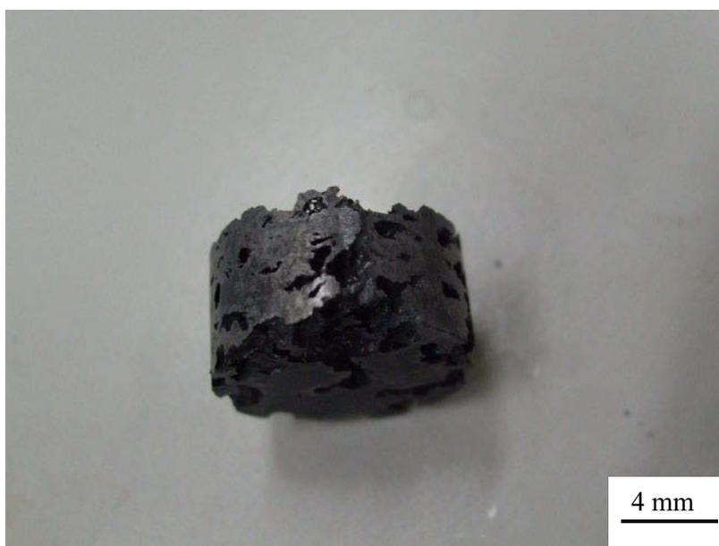
Fig. 1 Lead foam produced with SDP method from waste paste of a battery.
