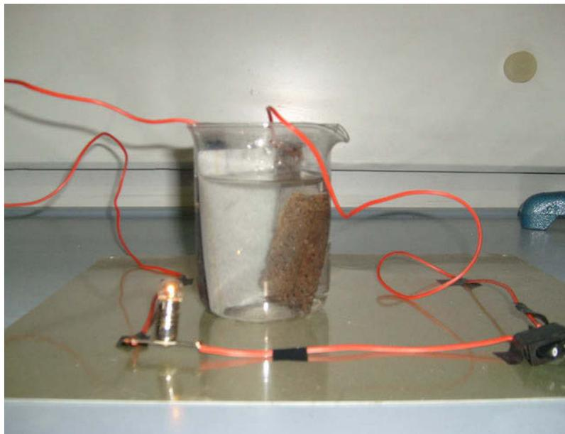
Figure 5. The 2V lead-acid cell with electrode foam charged and discharged.
