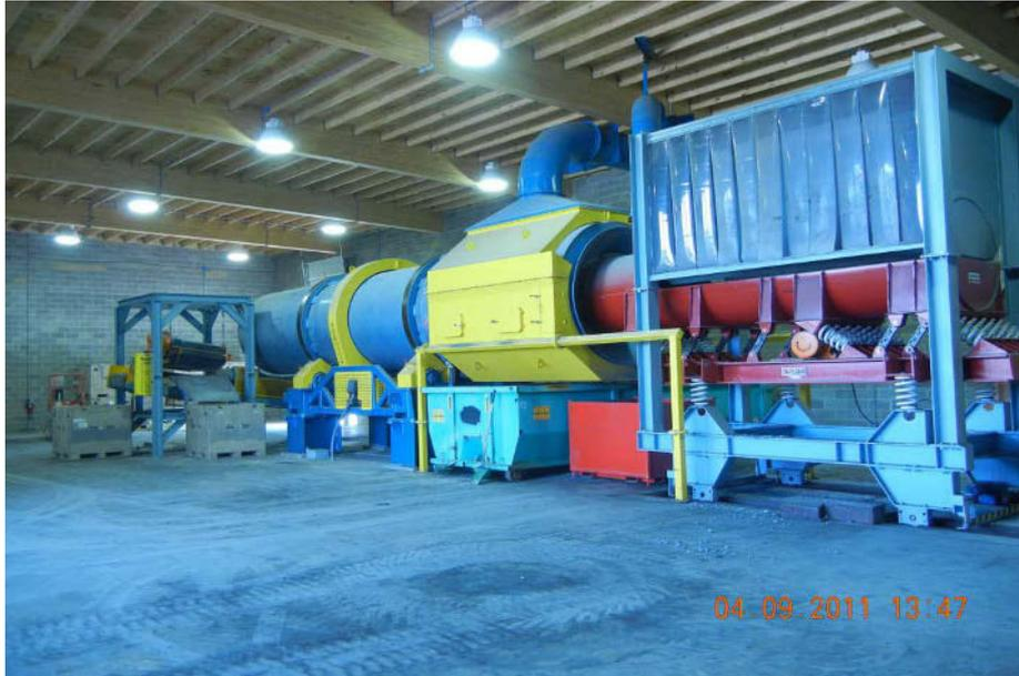
**Figure 5... DIDION RT 84 TUMBLER SYSTEM with Magnetic Separation.**
