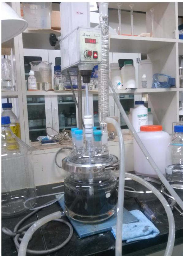
Figure 2. Experimental set up of the leaching process
