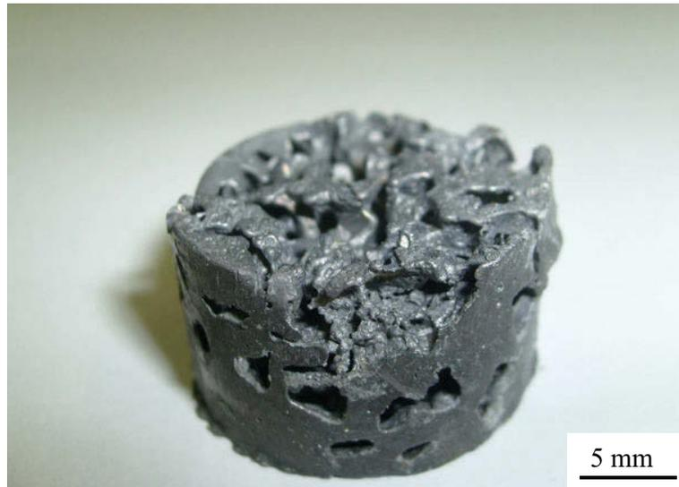
Fig. 2. Lead foam produced by RP process employing coarse NaCl as filler.
