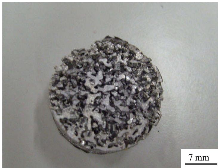
Fig. 3 Pb-Sn (60-40) produced by RP process employing coarse NaCl as filler.
