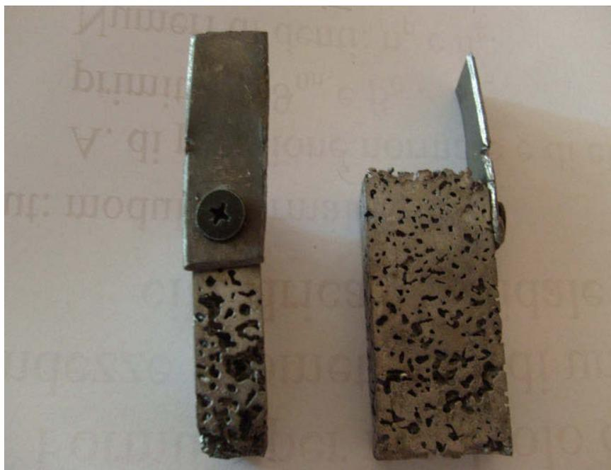
Figure 4. Rectangular cross-section lead alloy foams manufactured starting from grids of junk batteries.
