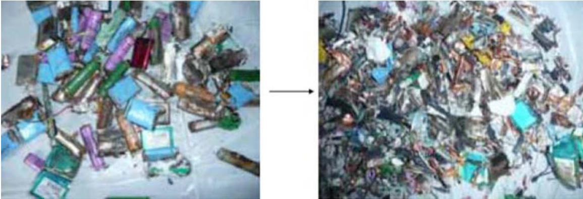
Figure 3. A lithium-ion battery before and after explosion in water.
