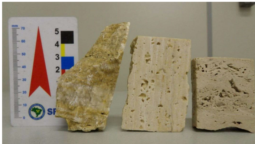
Figure 2 – Samples analyzed in Skyscan \mu CT scanner. From left to right: Itaboraí Travertine, Turkish Travertine and Roman Travertine.
