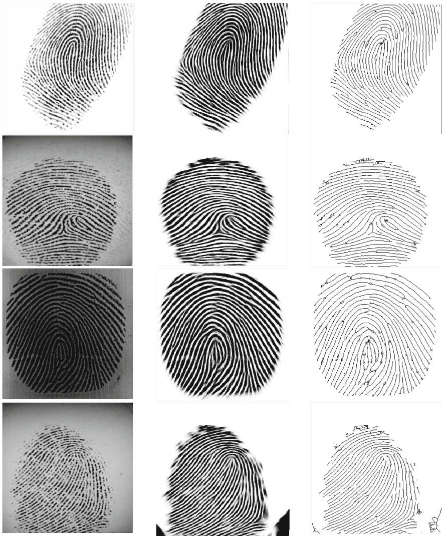
Fig. 5. Segmentation and enhancement results from FVC2002. Left column: Original image. Middle column: Results of rotational invariant anisotropic diffusion filter. Right column: Thinning and post processing. Row 1: FVC2002-DB1-A-9_3. Row 2: FVC2002-DB2-A-2_7. Row 3: FVC2002-DB3-A-4_3. Row 4: FVC2002-DB4-A-17_1
