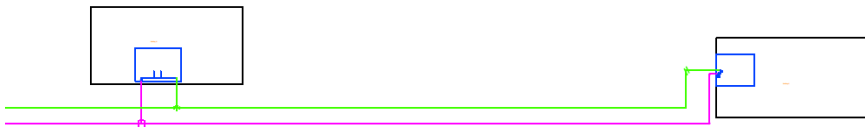
Fig. 6. Part of the supply and return pipelines for the primary circuit across buildings; where the purple lines are for the supply and the green line are for the return. And the blue lines are for the thermal bridge.
