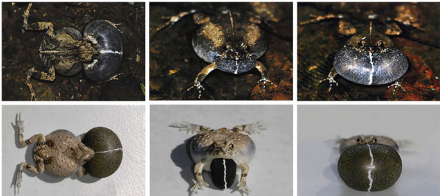
Fig. 11.4 Real and robotic versions of the túngara frog ( Physalaemus pustulosus ). Photographs in the upper row are of an actual calling male shown in different views and states of calling. Photographs in the bottom row are of a robotic túngara frog. The robotic frog has a dynamically inflating vocal sac that can be synchronized with its call (see Chap. 4). Modified from Taylor et al. (2008) and used with permission
