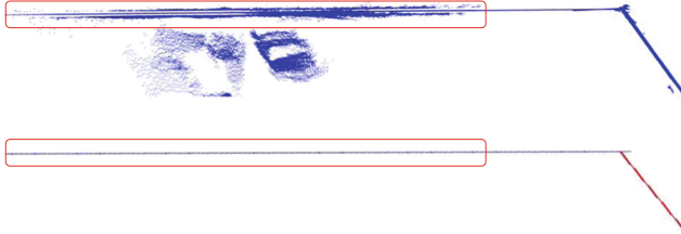
Fig. 5. Close overhead view of a planar region in the scene: (top) Raw point cloud representation and (bottom) 3D Plane-based map.
