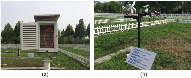
Fig. 5. Pyranometer and temperature sensor in AWS at UNIST. (a) Temperature sensor (HMP45D) in thermometer screen; (b) The pyranometer in AWS.
