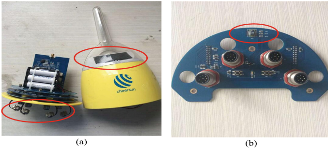
Fig. 6. Sensing node used in meteorological WSNs. (a) Interfaces on the bottom and solar cell panel in the shell. (b) On-board sensor SHT15 integrated on a circuit board.
