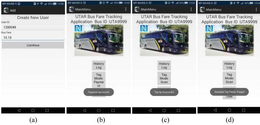
Fig. 6. mBus System (a) create new user (b) make payments (c) top-up (d) purging old pTag
