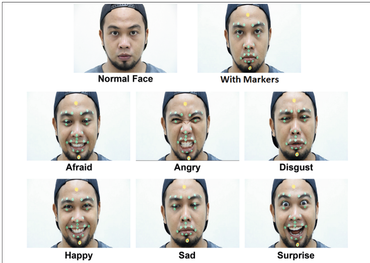
Fig. 2. Prepare a subject with markers at desired control points before facial performance. A total of 24 markers are used in this experiment. (Color figure online)
