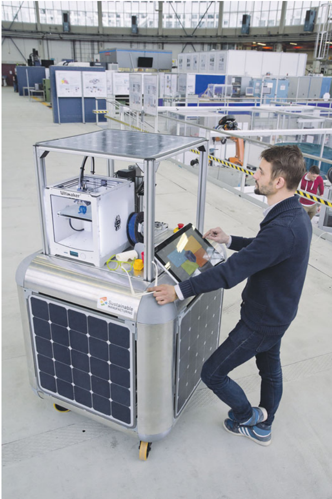
Fig. 6 CubeFactory: mobile, self-sufficient mini-factory
