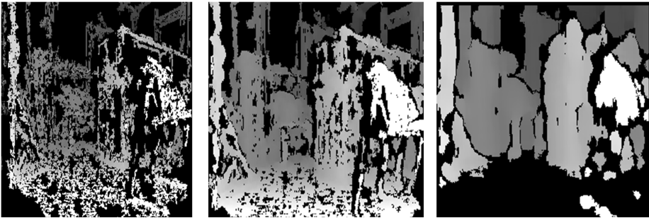
Fig. 3. Depth map from small (left), medium (middle), large (right) SAD window
