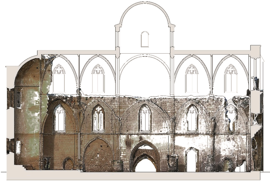
Fig. 3. A longitudinal section of the existing remains of the interior wall of the south aisle with a reconstruction based on proportional analysis of the arcuation of the nave, clerestory and cupola superimposed upon it.
