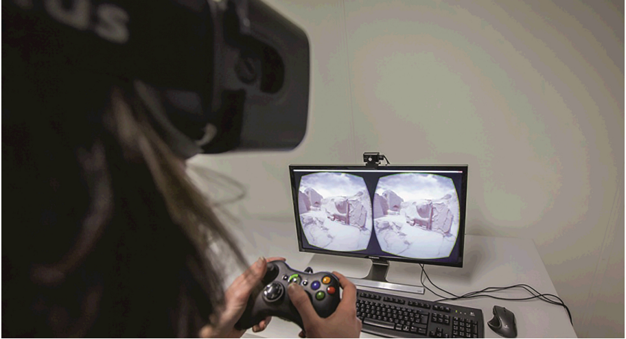
Fig. 2. The hardware setup used in the HMD application implemented in the virtual environment of the temple. The user wears an Oculus Rift DK2 HMD device. Movement in the virtual environment is controlled through a hand held Xbox 360 controller. The user's movements are captured through an external Oculus positional tracking camera positioned in front of the user.
