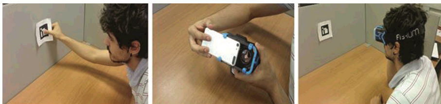
Fig. 3. Setting the marker and our HMD for marker based positional tracking
