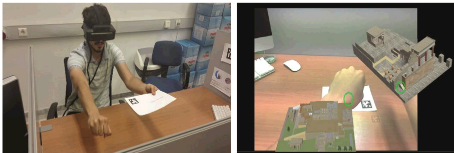
Fig. 5. Interaction using markers and hand gestures.
