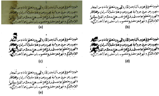
Fig. 2. Results (a) Original handwritten degraded image (b) Ground truth (c) Otsu's binarized image (d) Niblack's binarized image (e) Proposed approach binarized image
